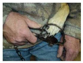
2. Compress the single long spring to relieve pressure to trap jaws. Use your feet if needed.
