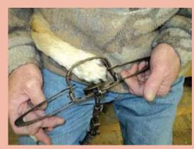
2. Compress both long springs at the same time to relieve pressure to trap jaws. Use your feet if needed.
