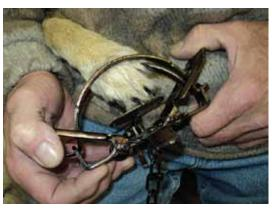
2. Compress both coil spring levers at the same to relieve pressure to trap jaws. Use your feet if needed.
